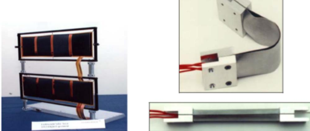
SMA Hinges for Solar Arrays
